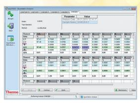
Typical operator analysis results screen with grade check
