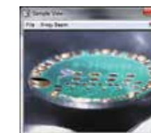
Camera view of a printed circuit board with the elliptical region of analysis shown at the center.
